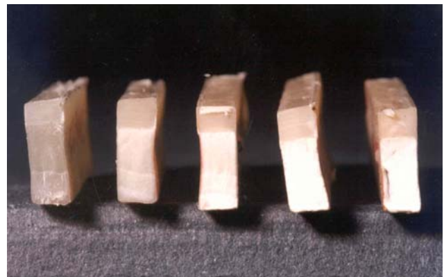
Fig. 4 Fractured surfaces of SAN/ NR-g-SAN blends at varying rubber content; From left C22/5, C22/10, C22/15, C22/20 and C22/25
